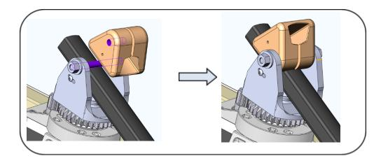
**Second step** : The pivot is now link to the support arm although it can move. The pivot will be completely located in the assembly when the link between the pivot and the detector will be done.
